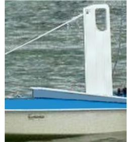
**CENTERBOARD** – A rotating wood or fiberglass **keel** used to stabilize a *midsized* sailboat. It is secured in the **center** of the hull and can be rotated or **pivoted** down in deeper water. It may be brought up in shallow water or when sailing downwind.
