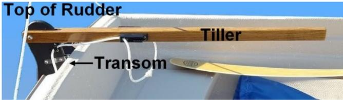
**TRANSOM** – A vertical, flat surface at the back or **Stern** of the hull, where the rudder and/or motor are attached.
