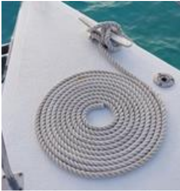
Left: A Dock Line in a Flemish Coil and secured to a Deck Cleat Right: Deck Cleat on top, Cam Cleat on bottom
