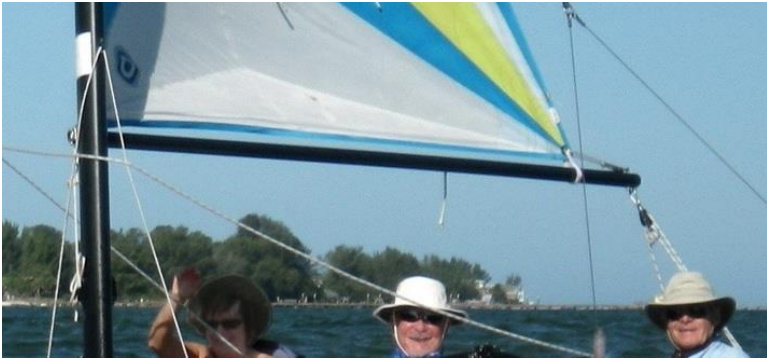
The Boom is connected to the Mainsheet (see block and line on right)
