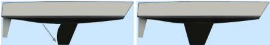
Fig. 8. Centerboard (left), Keel (right): dark bottom of boats above
